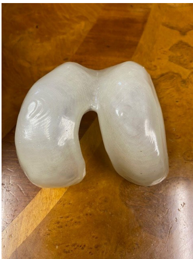
The images here show the effects of vapor smoothing of the iKnee implant after its initial 3D printing. This process provides the optimal surface for providing durability and comfort as the cushion for the distal femur's movement in the knee joint.
