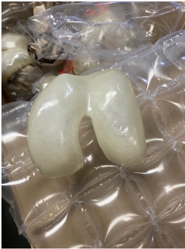
The images here show the effects of vapor smoothing of the iKnee implant after its initial 3D printing. This process provides the optimal surface for providing durability and comfort as the cushion for the distal femur's movement in the knee joint.
