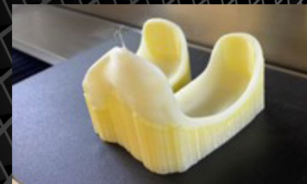
The very first PFD/iOI printed iKnee with the support material rolls out picture perfect.
