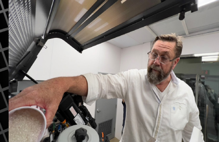
Eric Hansen, PFD Co-founder and Patient One, loads the Quadrathane into the Arburg.
