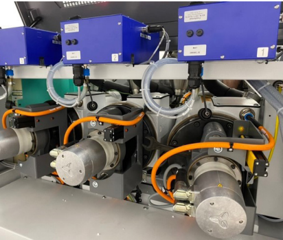
Injection is individually controlled by three separate motors.
