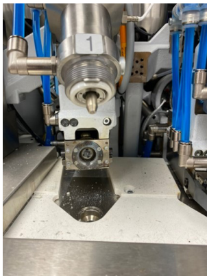
Print nozzles provide precision controlled material injection.
